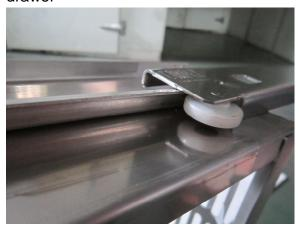
C. Lift drawer and remove from channel.
